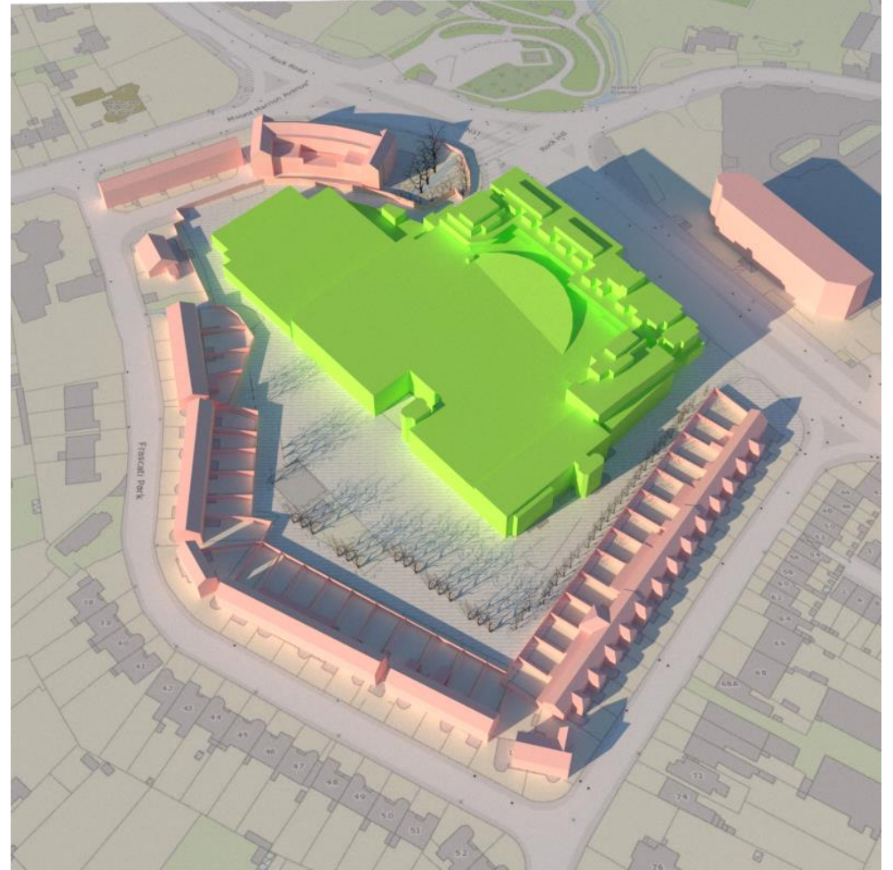
Shadows Cast at 4pm (UTC+0) on the 21 st March - After Development Scenario
